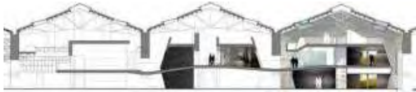
Transparent surfaces on the roof: solar gains
