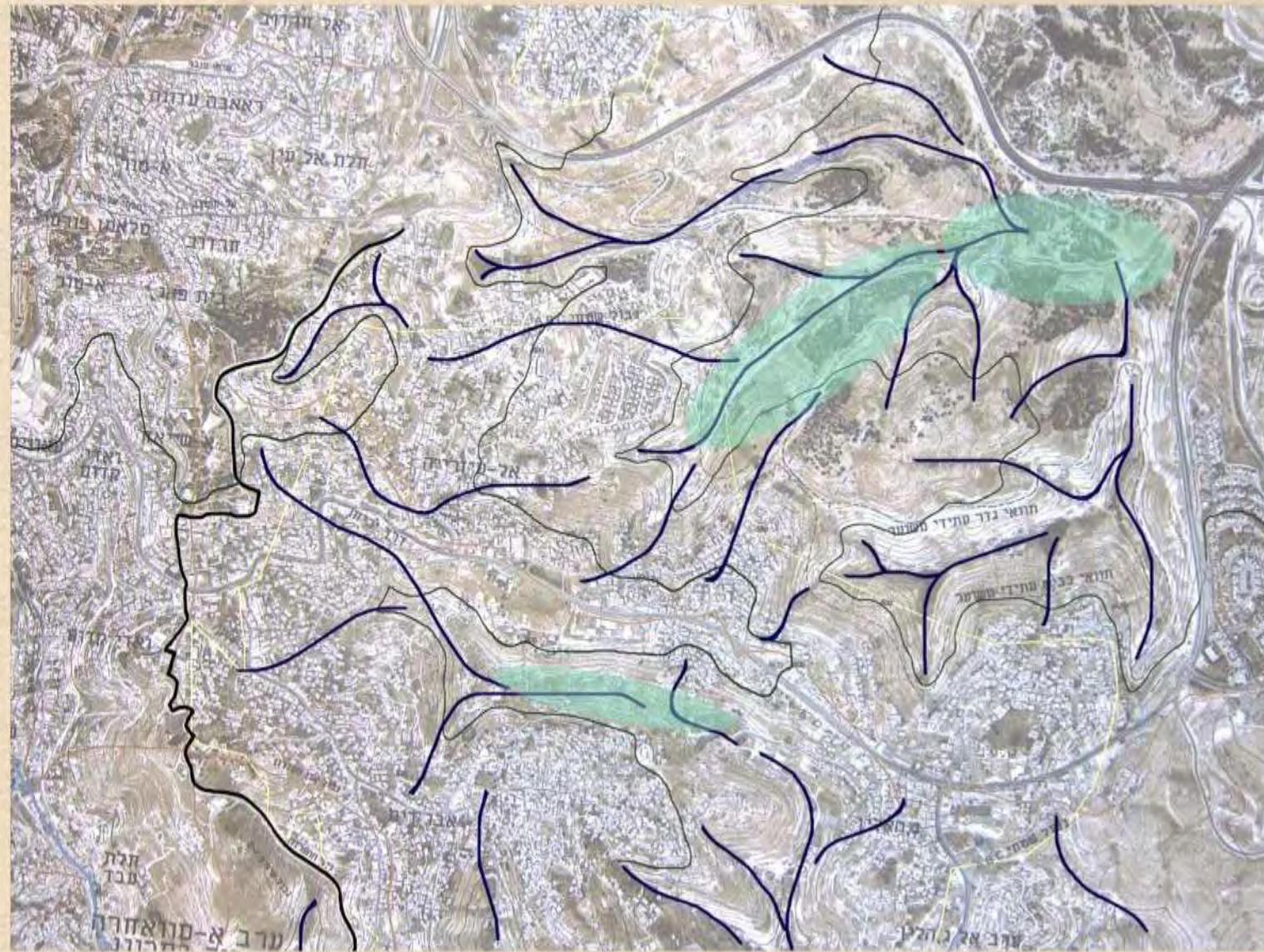
Flow of the rain water and points of collection
